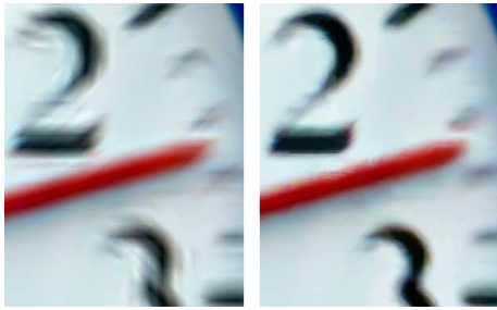
Figure 8: Artifacts reduction obtained with the iNEDI method(right) with respect to NEDI (left): non local effects are clearly reduced by adapting window shapes and size, discarding high frequency interpolated values and optimizing the least squares procedure.
