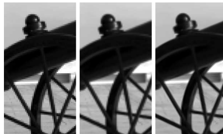
Figure 5: 8X enlarged images. Jagged contours are evident in nearest neighbor and bicubic interpolation (left, center). The NEDI interpolation (right), present sharp edges, even if introduces different artifacts and perform often worse than the bicubic method in quantitative comparisons. Our improvements to the method reduce evidently these effects.
